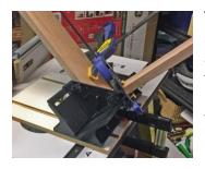
**Tom** fabricated the cabinet box frame using splined miter joints, employing his router table and a **Rockler Router Spline Jig** – noting that the large size of the frame made for an awkward routing situation! One quarter inch walnut splines, which contrasted nicely with the oak frame, provided additional joint reinforcement.
