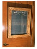
In addition, the whole cabinet was designed to be securely attached to the outside of a closet door, using hangers affixed near the top of the back panel and rubber bumpers along the bottom of the panel to prevent marring the finish of the closet door.
